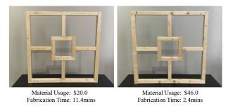
Fig. 11. Fabrication results of two window variations. The different designs and fabrication plans trade-off fabrication time and material usage.
