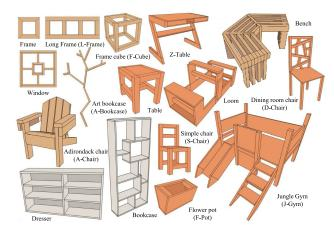
Fig. 7. Models used for all experiments in Section 5. Brown is used to indicate the models which are only made from 1D sequential cuts of lumber. Gray is for only from 2D partitioning of sheets. Orange is for both using 1D sequential cuts of lumber and 2D partitioning of sheets.
