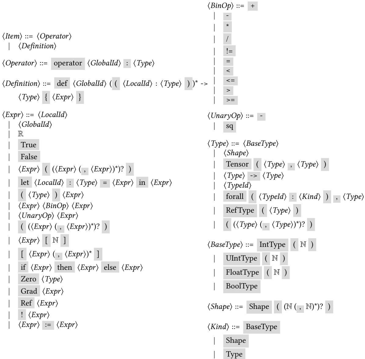
Figure 3. The BNF Grammar for the Relay language. Each case matches a node in our abstract syntax tree. References and related operations cannot be included in frontend user code and are only generated by the reverse-mode automatic differentiation.
